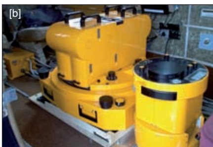
Fig. 1 (a) - The Carl Zeiss Jena MFK-6 multi-spectral film camera that was used on various Soviet spacecraft had six lenses and six separate film magazines. (Source: Deutsche Museum) (b) - The Carl Zeiss Jena MSK-4 four channel airborne multi-spectral film camera on its mount with its viewfinder and navigation/tracking device at the right. (Source: MGGP Aero) (c) - A Carl Zeiss Jena LMK-1000 photogrammetric film camera mounted in a Piper Navajo aerial photographic aircraft. (Source: MGGP Aero)
