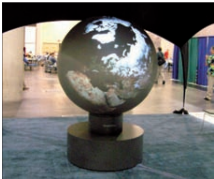
Arc Science Simulations presented an innovative visualization monitor. Their 1-meter diameter globe projector is able to show all kinds of map data in a realistic view 'as the world turns'.
