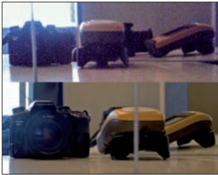
Part of an image taken with the internal camera (1.3 MP) and a similar image using a semi-professional 6 MP camera. Both images have been edited and scaled in a similar manner and are directly comparable.
