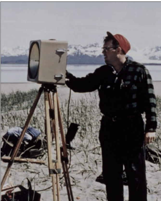
The Tellurometer was one of the first electronic positioning systems used in land survey (source: www.photolib.noaa.gov ).
