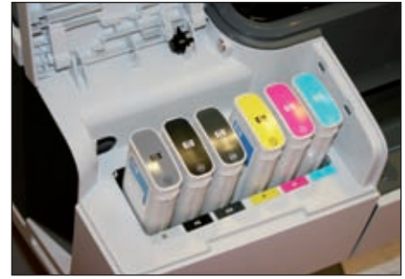
The six Vivera inks in the T-series, including matte black, photo black and grey.
