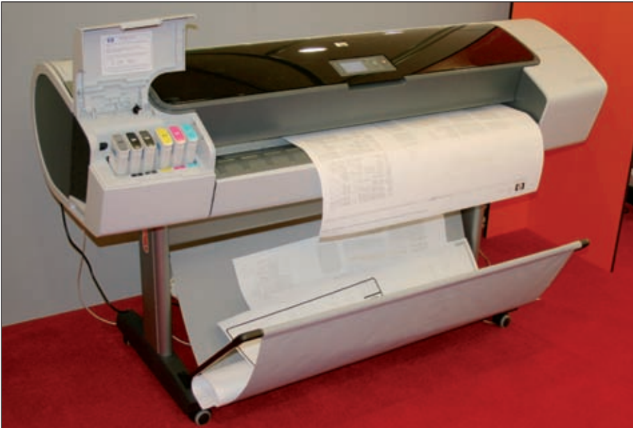
HP Designjet T1100 line accuracy is improved at 0.1 per cent.
