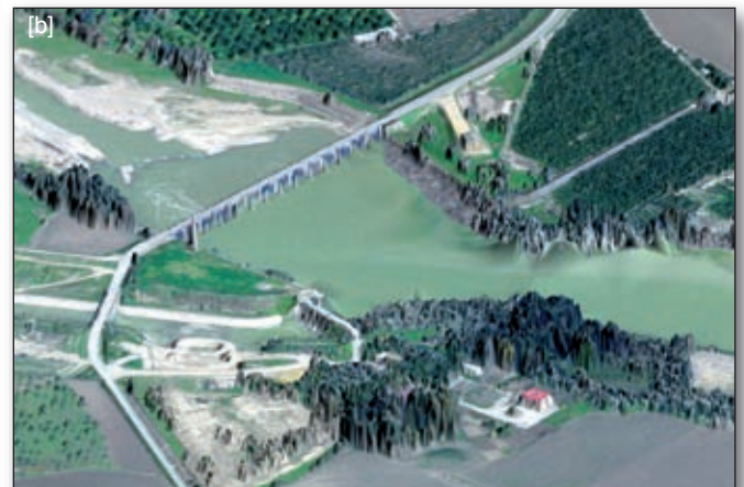
(b) - A 3D perspective view of the same area produced by merging the orthophoto image data with the elevation data acquired by an Optech ALTM-3100 airborne laser scanner.
