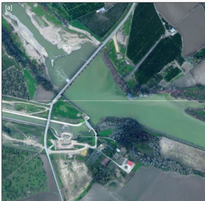
Fig. 7 (a) - An orthophoto image showing a part of the valley of the Guadalquivir River in Andalusia, Spain produced from airborne digital frame images acquired by a Rollei AIC camera.
