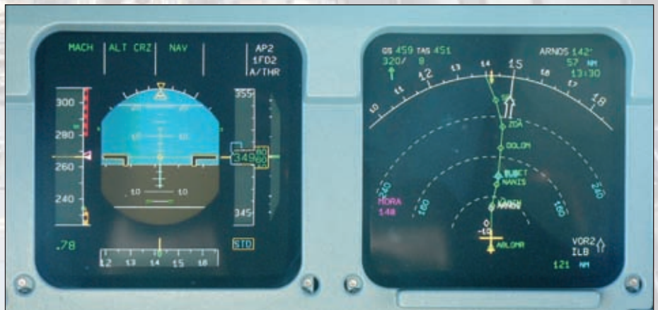
Detail of the Primary Flight Display on the left and Navigation Display. Flying on 35,000 ft, speed 0,78 Mach. Arnos is the active waypoint, the route is over Austria with Zagreb (ZDA) and Split (SPL) on the way.
