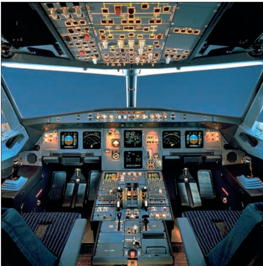
The cockpit of an Airbus 320 with the Navigation Display in the middle, left and right. The two Control and Display Units a little lower an almost next to each other and the IRSs top left. The importance of GPS in aviation is increasing. Source: www.airbus.com
