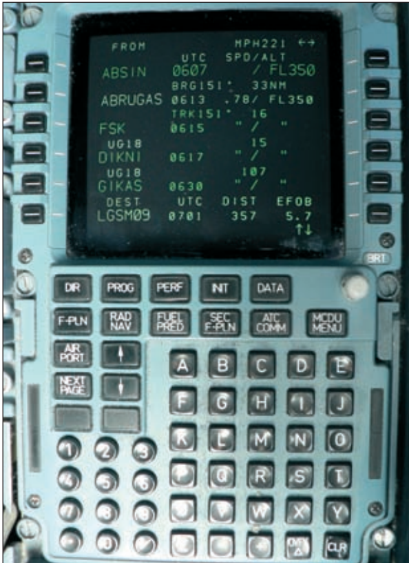
Close up of a Control and Display Unit, on the display a part of the flight plan.
