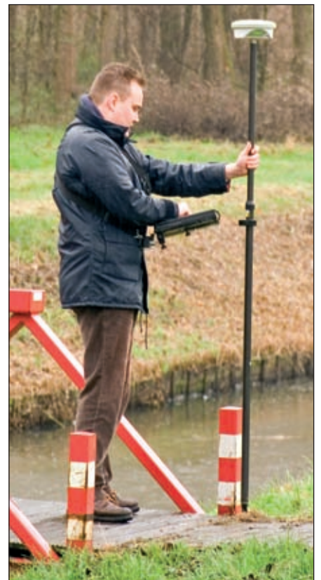
Measuring a survey point using a Tablet PC
