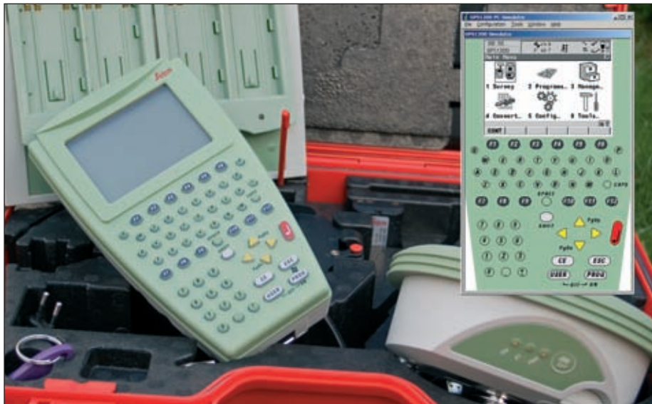
Complete Leica SmartRover set as tested. Inset is software controller from Leica MobileMatriX
