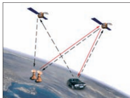
The central control system sends inquiry signals to the users via two satellites. Source: www.globalsecurity.org
