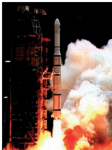
The launching of a CZ-3A that is used for getting the Beidou satellites in orbit.
