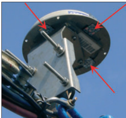
Using retro-reflection stickers on the rim of the antenna will ease the location determination with conventional land survey techniques.
