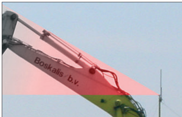
Figure 1: shielding caused by a backhoe boom.
