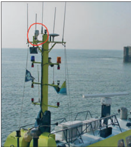
Installation on a survey vessel. The antenna is installed in the top of the mast.
