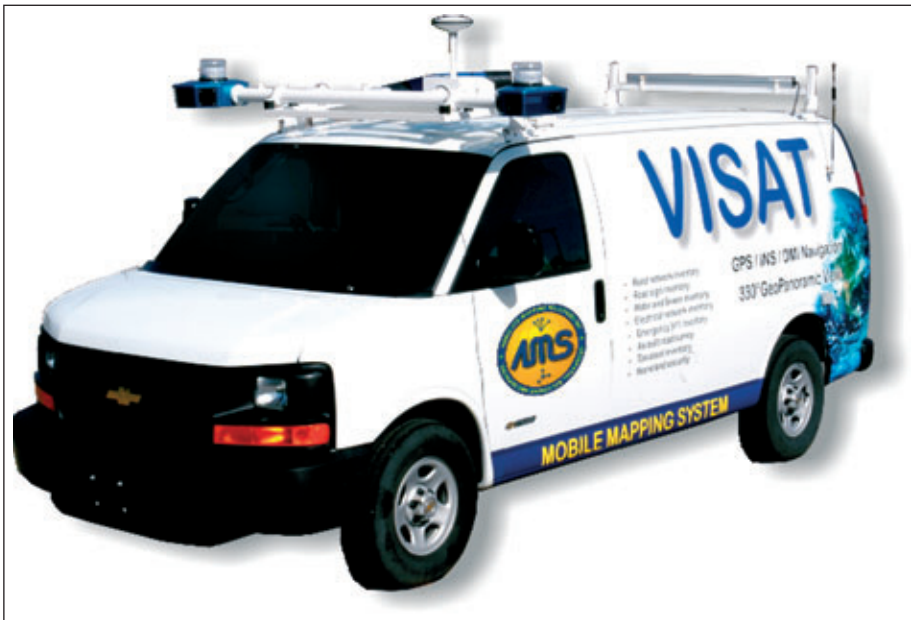
Figure 3: The VISAT Van from Absolute Mapping Solutions.
