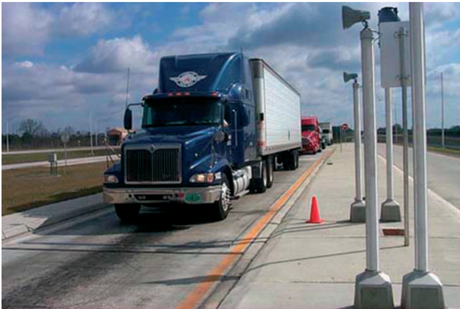
Figure 6: One ORNL application involves chemical and radiation sensors at truck weigh stations. (Photo Metler Toledo.)
