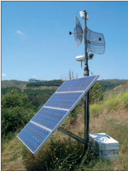
Bijlschrift: Figure 2: Solar powered wireless weather station. (Photo San Diego State University Field Station Programs.)
