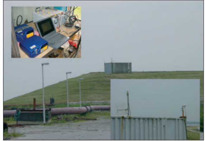
Permanent station. Potential problems with this set-up: multi-path and shifting. The first was remedied by a ground plane, the second by regular resurveys.
