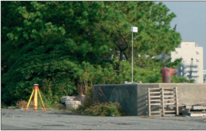
This temporary station is located too close to the tree line to achieve optimum results. (source: www.nmri.go.jp )
