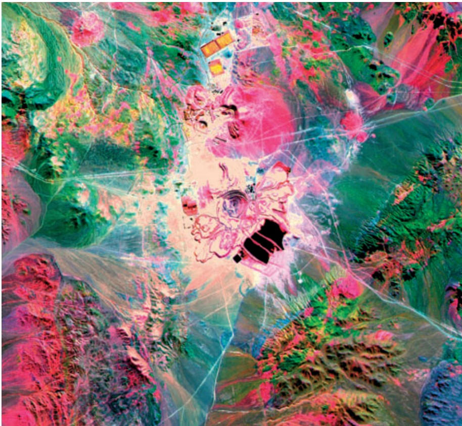
Figure 3: Aster Image with SWIR bands 4-6-8 in RGB, and highlights lithologic and alteration differences of surface units. (Courtesy: http://asterweb.jpl.nasa.gov/gallery-detail.asp?name=Escondida )
