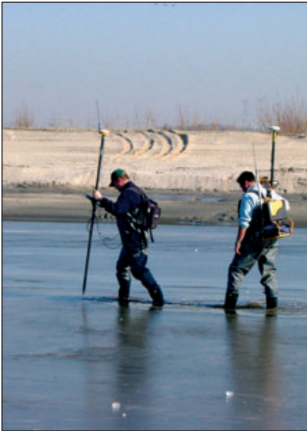
Two land surveyors using RTK backpacks and separate GPS antenna.
