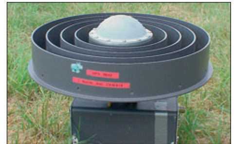
Figure 5: antenna with choke ring to prevent multipath (source: www.ipgp.jussieu.fr ).
