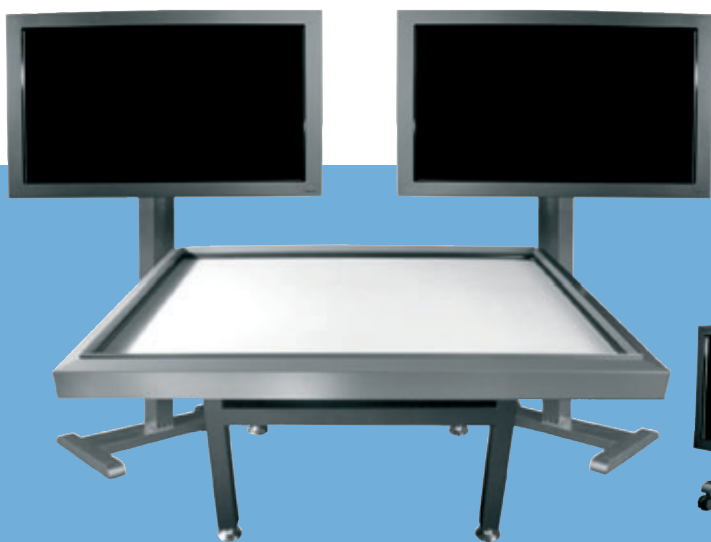
(a) The TouchTable TT84 with its 84 inch (213cm) diagonal table is equipped with a matt-white powder-coated aluminium display surface that responds to hand (or finger) movement and pressure. The TT84 sits on a tubular steel frame equipped with levellers. This particular example also features two 50 inch (127cm) diagonal touch-sensitive plasma displays mounted on stands in a vertical position alongside the main table.
